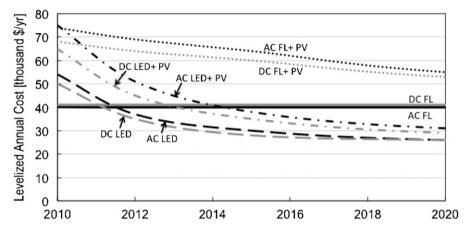
**Fig. 4.** 2010–2020 LAC projections for grid-connected AC vs. DC fluorescent and LED lighting systems. Results do not decline significantly between 2020–2030 and are excluded from the figure. The electricity price assumed is \$0.10/kWh, and the discount rate is 12%. LED projections are from DOE R&D targets (2011b) and solar PV projections are from Curtright et al. (2008). These results assume that DC circuits eliminate the need for LED drivers and a PV inverter.
