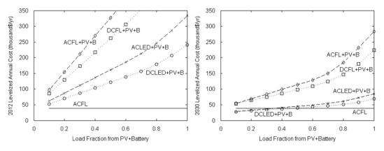
Fig. 7. 2012 and 2030 lighting system LAC projections vs. fraction of load provided by solar PV and batteries
