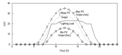
**Fig. 2.** Load profiles for LED Lighting system vs. solar PV output in Pittsburgh, PA. Load profiles generated from PV-integrated DC LED lighting systems with 100% of the load electricity requirements (on average over the year) provided by PV and energy storage. *Sources*: (NREL, 2010; NOAA, 2010).
