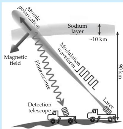
frequency in the magnetic field. The researchers calculate that such a system would achieve subnanotesla sensitivity and could lead to the formation of a global network for continuous mapping and monitoring of mesospheric magnetic fields. (J. M. Higbie et al., *Proc. Natl. Acad. Sci. USA* **108**, 3522, 2011, doi:10.1073/pnas.1013641108.) —JNAM
