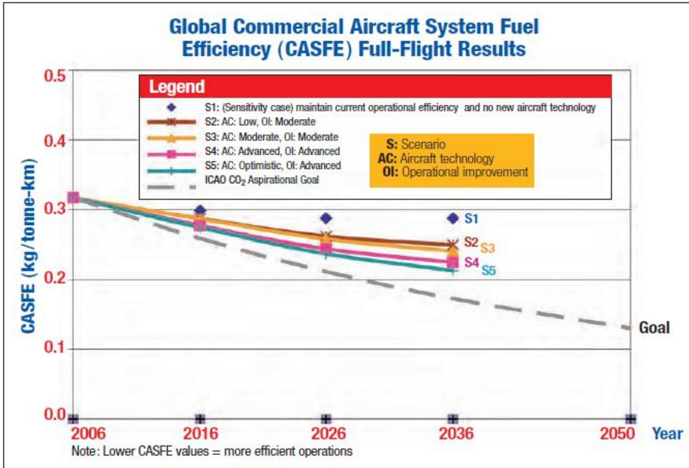
Figure 4: Commercial Aircraft System Fuel Efficiency (CASFE) Full-Flight Results.
