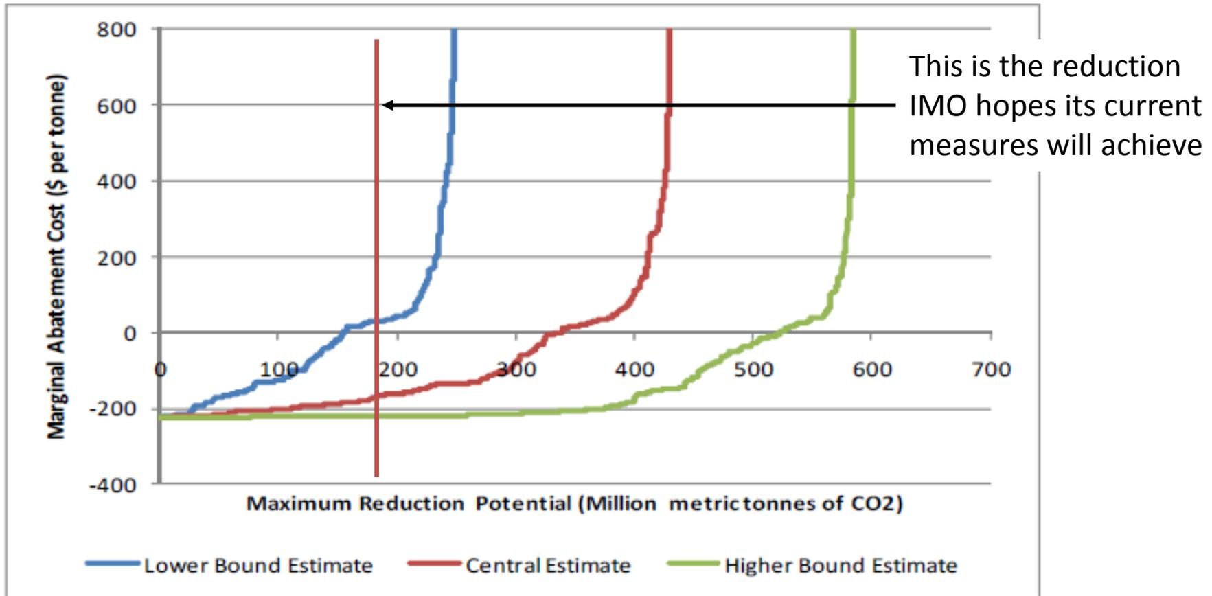
Figure 6-1: Aggregated MACC in 2020 with \$700 per ton fuel price and 10% discount rate for all ship types.
