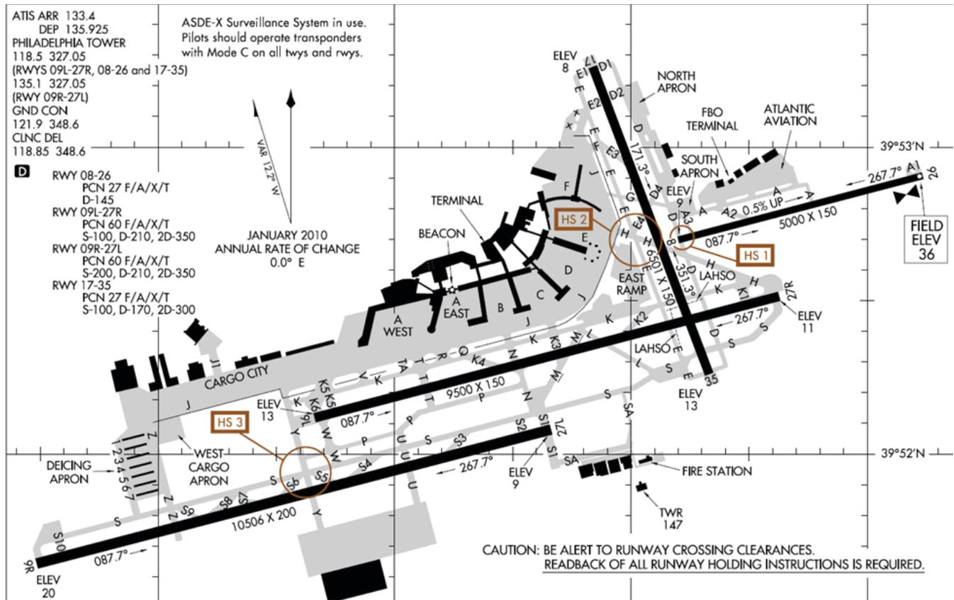
FIGURE 7 Layout of Philadelphia International Airport allows aircraft departing eastward from Runway 9R to exit departure queue and decouple from tug at deicing apron (circled at lower left).
