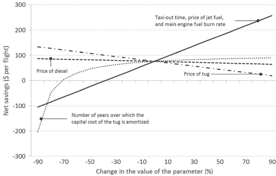
FIGURE 4 Sensitivity analysis showing impact of various parameters on average net savings.
