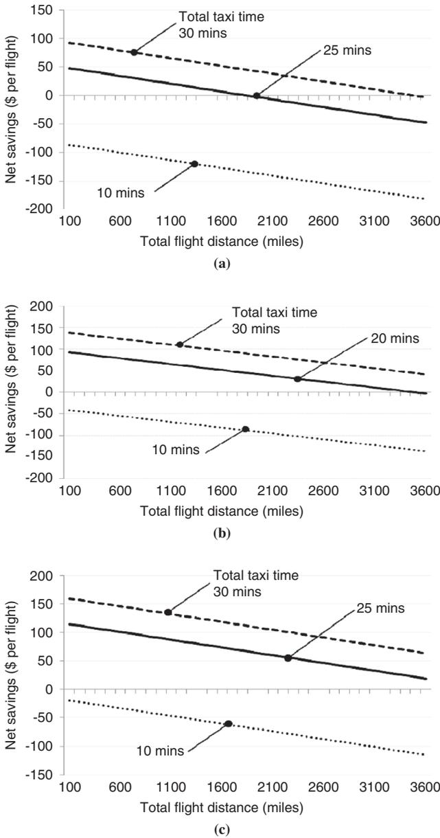
FIGURE 6 Net savings versus total flight distance for various total taxiing time and capital costs per A320 aircraft of (a) \$1 million, (b) \$500,000, and (c) \$250,000.
