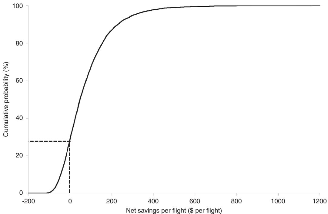
FIGURE 2 Even at service level of 65%, about 30% of flights departing from Newark would lose money if towed by tugs. Towing flights that do not taxi for long would reduce savings, whereas towing flights with long taxi times would increase savings.
