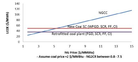
FIGURE 2. Levelized Costs of Electricity for Retrofitted and New Plants
